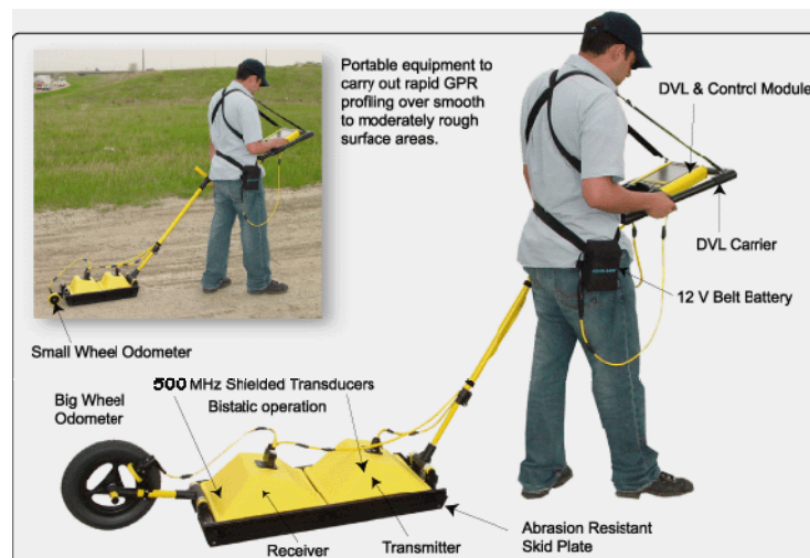
Fig. 3: The GPR system used in these archaeological investigations.
